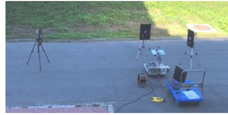
Fig.6 Arrangement of LED landmarks
