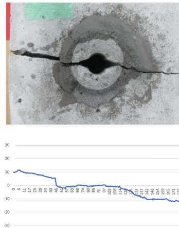
Fig.4 crack of specimen and digitized graph
