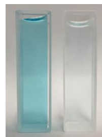
Fig. 4 Change in color of methylene blue aqueous solution after adding HCl without (left) or with (right) bubbling for 3 hours (right)
